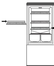
Ensure that foods does not touch the back wall. The trays have a limit point for this purpose which should not be exceeded.
