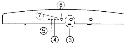
Turn the thermostat ③ control clockwise to turn the pilot ④ off and start the freezer. The alarm ⑤ also comes on because the freezer is not yet cold.
