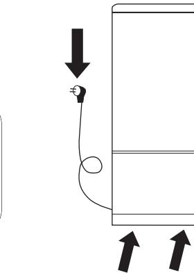
**IMPORTANT.** Ensure that the refrigerator is well seated on the ground (without movement) and is properly levelled (without tilting) by adjusting the levelling feet.
