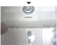
\* Pull down R-light cover a little to separate the hook and pull out forward smoothly.
