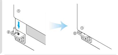
2 Let the top of door close to the cabinet and insert the top hinge pin to the top hole of freezer door.
