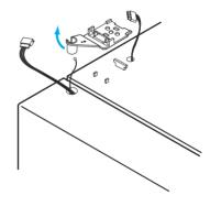
Lift the door straight up to remove.
