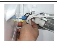
\* Seperate F-lights housing & Heater housing (Eva front cover) from the interior side terminals.
