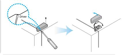
Turn top hinge fastener counterclockwise 3~4 times.
