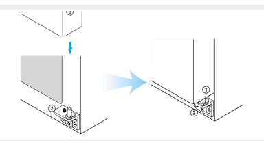
Let the top of door close to the cabinet and insert the top hinge pin to the top hole of freezer door.
