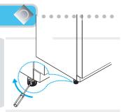
Open the doors, unscrew the front cover and remove, if it is attached.
