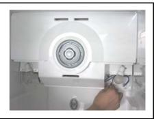
\* Unscrew two screws on the left and right side of DAMP COVER.
