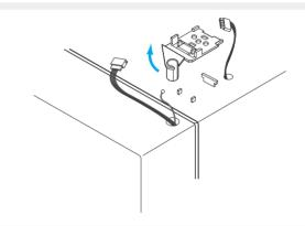
✓ Lift the door straight up to remove.
