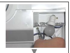
\* Hold the bottom and right of damper to pull down to remove.
