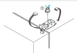
Lift up the front of hinge to remove. (After the hinge is removed the door can fall down forward. Be careful!)
