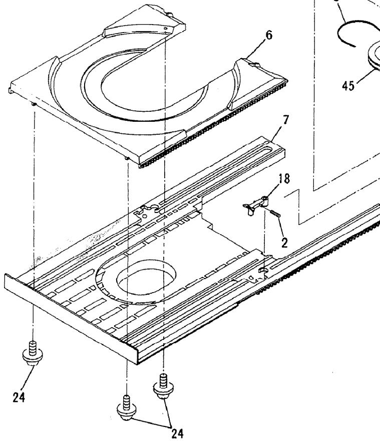
• Servo mechanism assembly T
