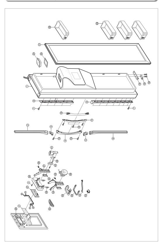
14-7) Freezer Room Door Exploded View (SR-S2028, S2029, S2228, S2229/S20DTC,S20FTC,S22DTC,S22FTC)
