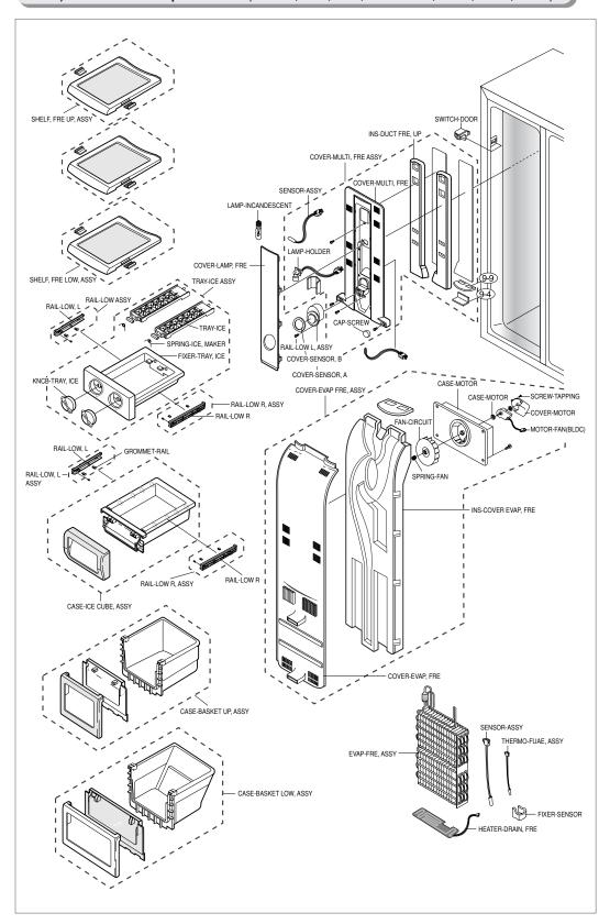
14-1) Freezer Room Exploded View (SR-S2026, S2027, S2226, S2227/S20NTC, S20BTC, S22NTC, S22BTC)
