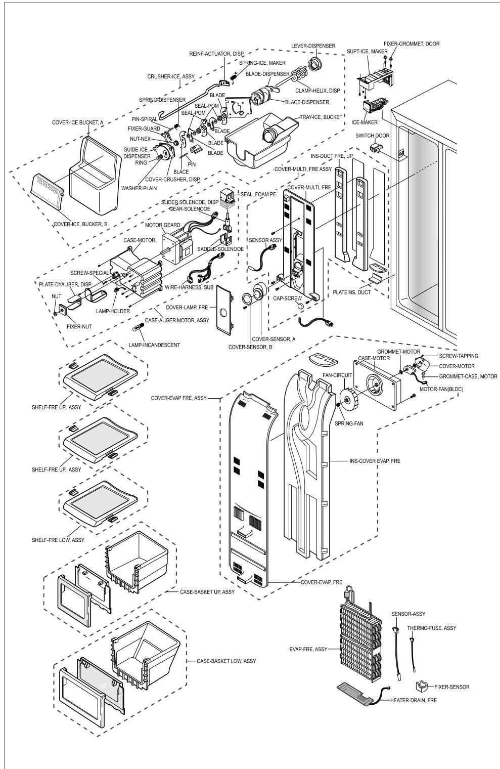
**14-5) Freezer Room Door Exploded View (SR-S2026, S2027, S2226, S2227/S20NTC,S20BTC,S22NTC,S22BTC)**
