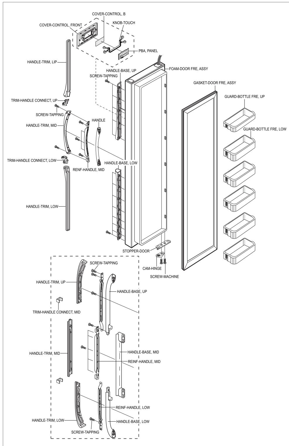
**14-6) Refrigerator Room Door Exploded View (SR-S2026, S2028, S2226, S2228/S20NTC,S20DTC,S22NTC,S22DTC)**
