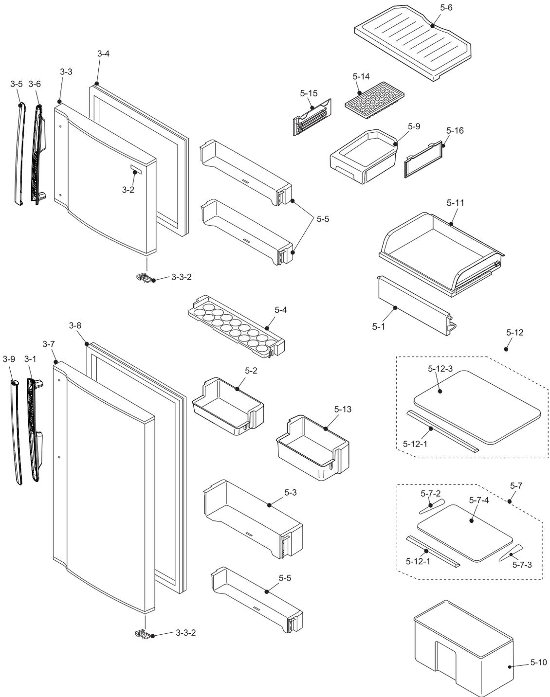
[5] SJ-380V/420V-SL/WH/BE ELECTRIC,MECHANICAL,CYCLE PARTS
